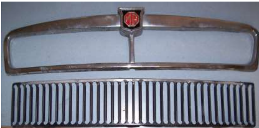
Later grille (Mk I & II). Grille made of pressed aluminium.
