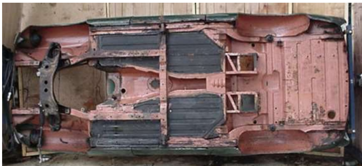
Photo showing monocoque construction (photo: mg.net)
