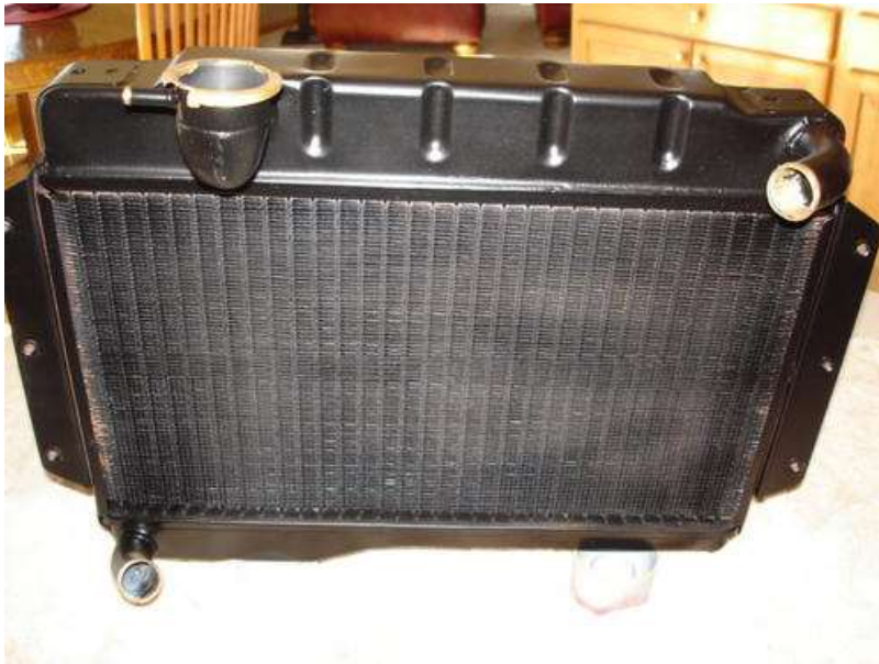
Early style radiator with refill access to the left
