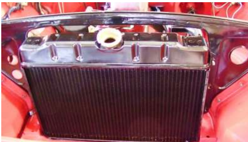
Later style radiator with central refill access
