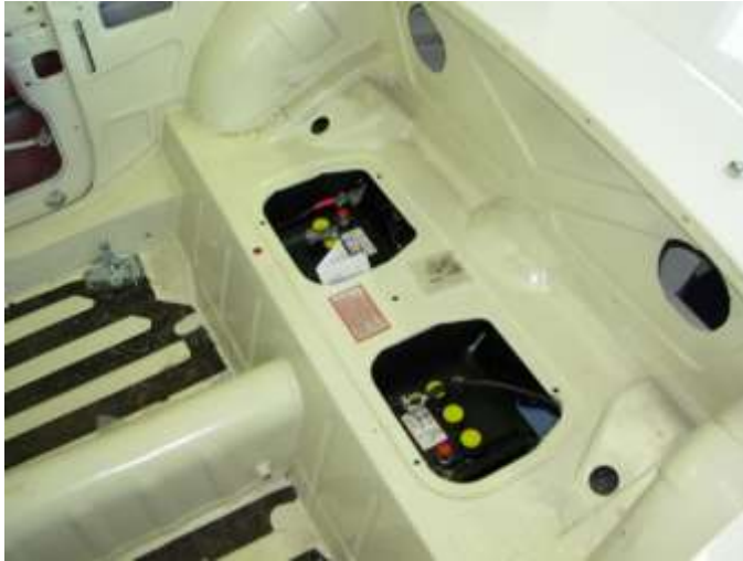
2x 6 volt batteries under rear compartment
