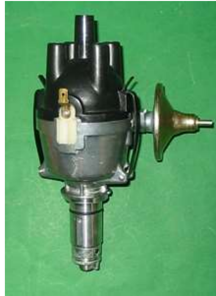
Lucas 25D distributor showing early side exit (18G,GA & GB) and later (18GD-) top exit
