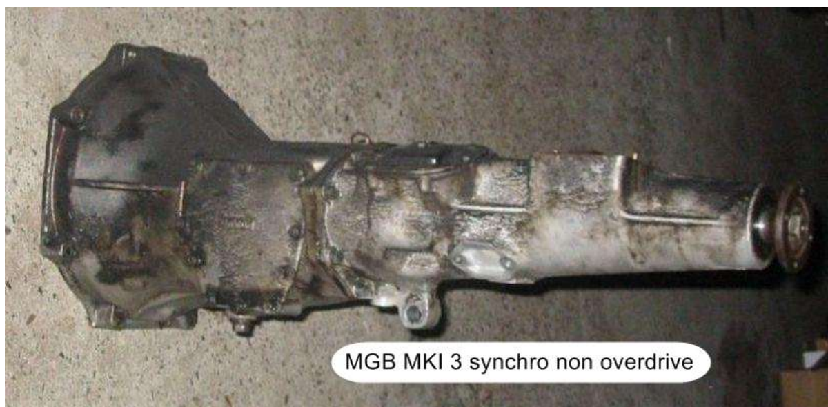
Mki-3 synchro/no overdrive (photo MG Spare Parts & Services)
