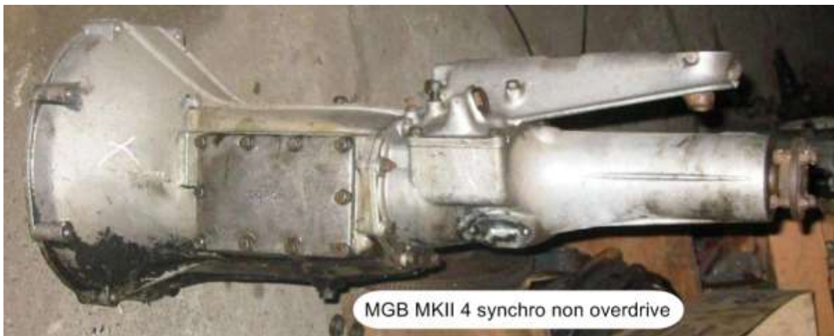
MkII-4 synchro, no overdrive (photo: MG Spare Parts & Service)
