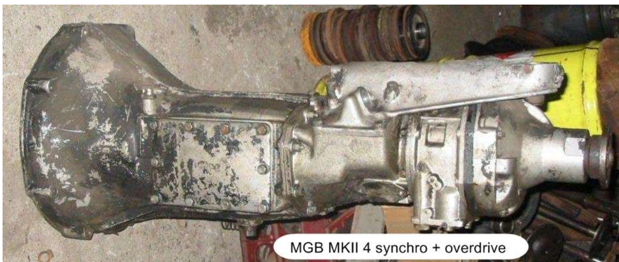
MkII-4 synchro + overdrive (photo: MG Spare Parts & Service)
