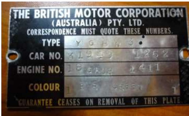
Early 'Enfield' plate. Note: additional numbers are UK chassis numbers and stamped from the front
