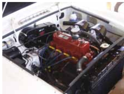
Almost completed engine bay; bonnet cable P clips and spark plug leads still to do.
