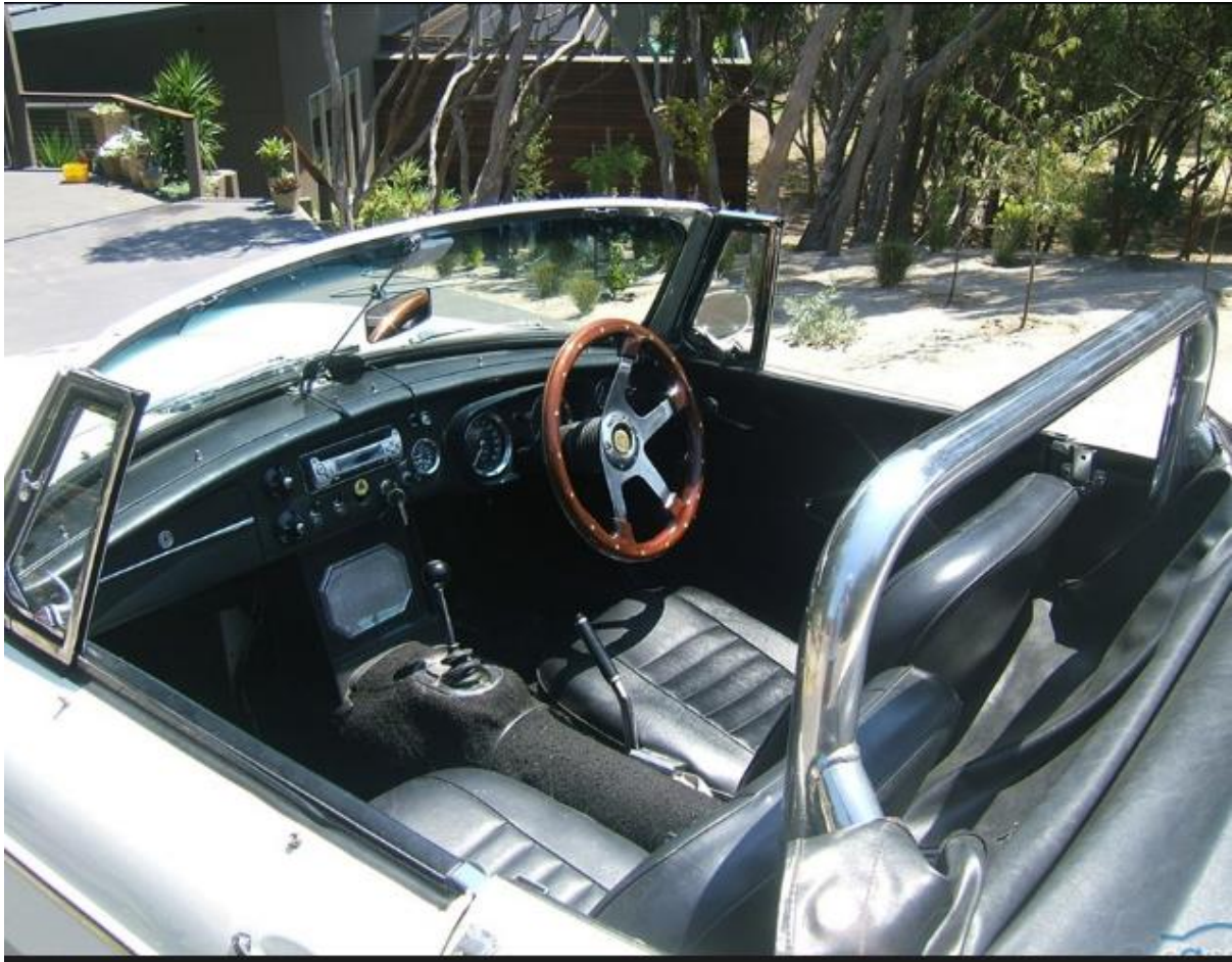
Narrow gearbox tunnel on YGHN3/5166 (note the hump below the gear lever and the overall narrowness of the tunnel)
