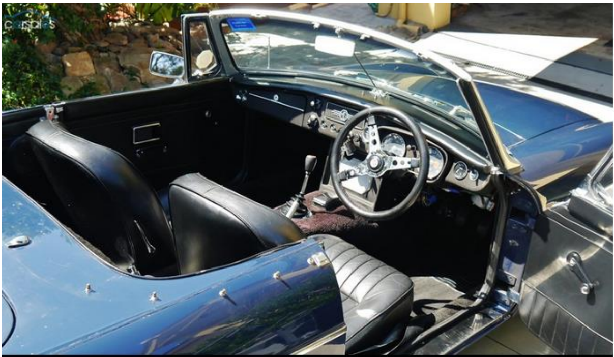
1968 Wide tunnel on a YGHN4 (note that the hump has gone and the tunnel is flatter and wider)
