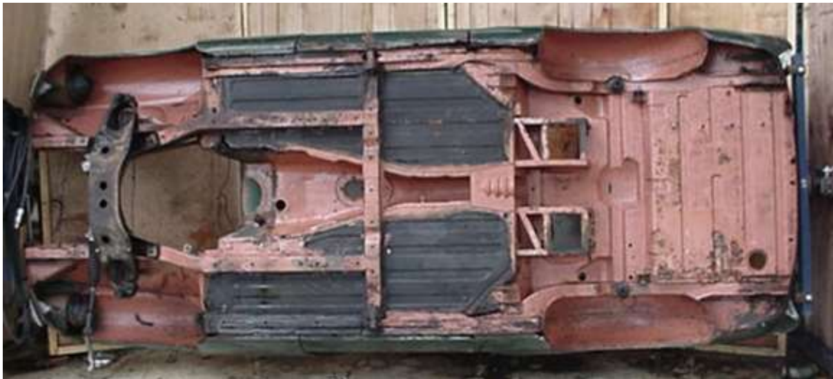
Photo showing monocoque construction (photo: mg.net )
