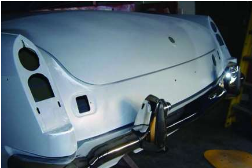
This photo shows the pressings made for the reverse lights (photo: A Helgeson)
