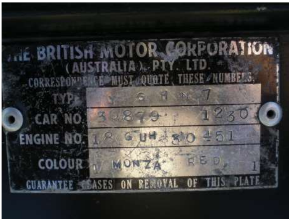
This YGHN3 car was incorrectly stamped YGHN7
