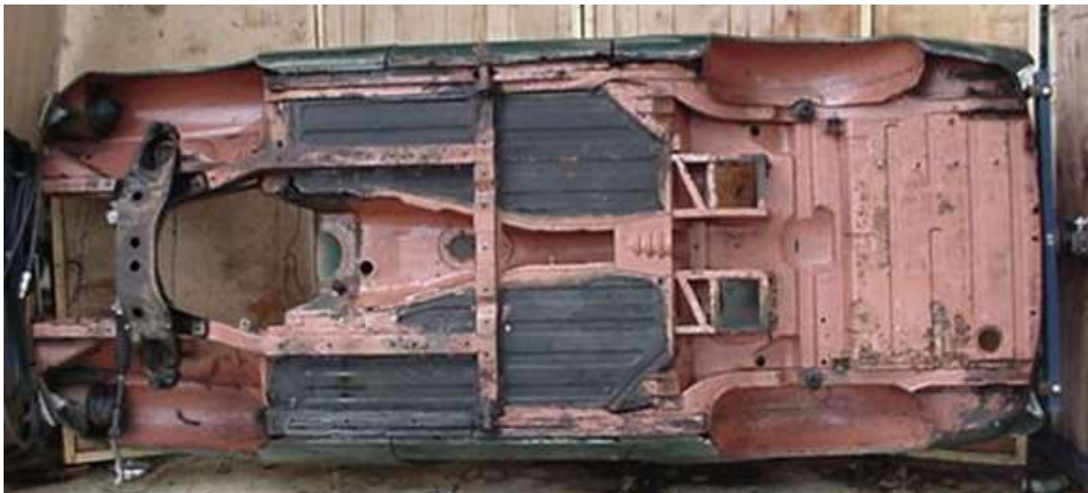
Photo showing monocoque construction (photo: mg.net)
