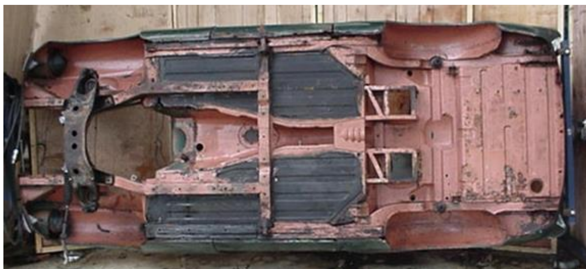
Photo showing monocoque construction (photo: mg.net)
