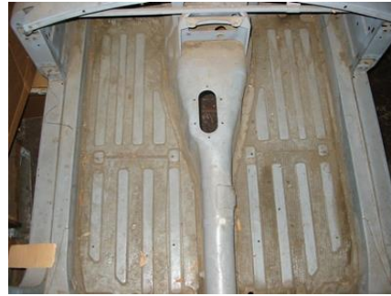
Figure 1 Early 3-sync tunnel c/f wider 4-sync tunnel. Compare the ribs on both sides to see the difference
