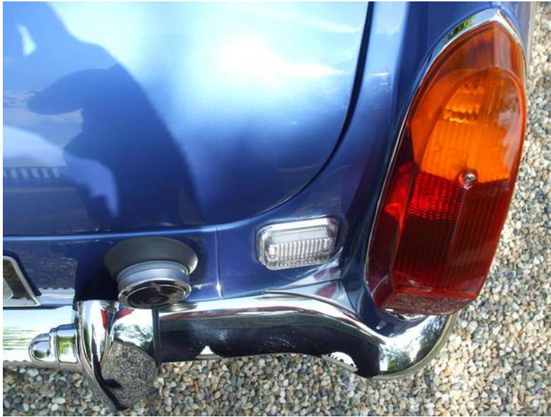
Later smaller bumper infill (polished alloy)
