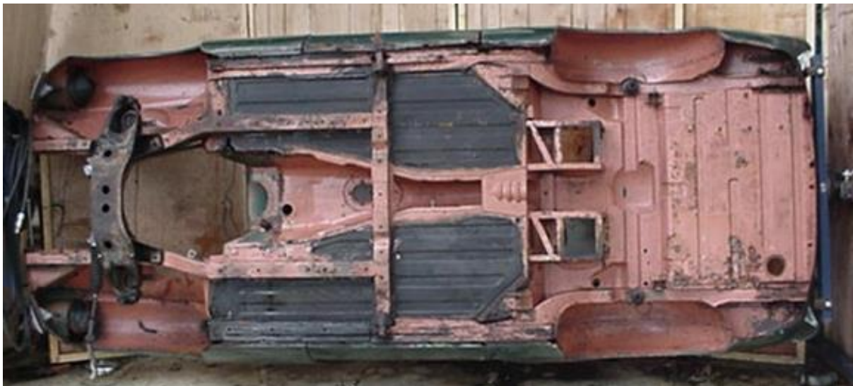
Photo showing monocoque construction (photo: mg.net)
