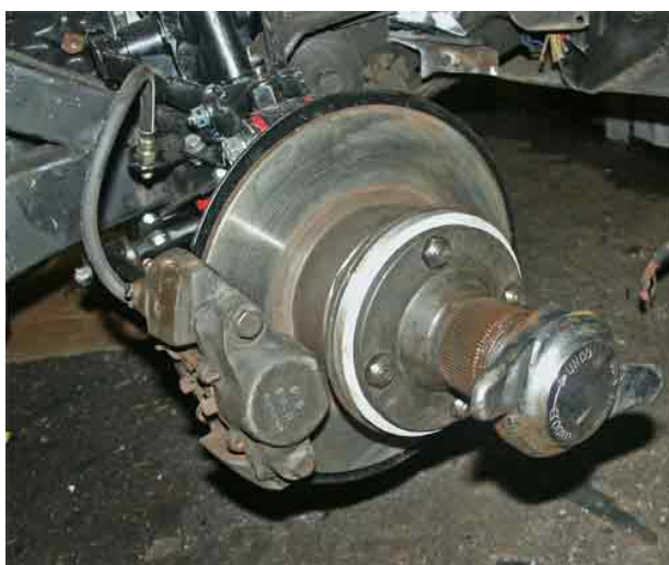
Right front disc brake assembly
