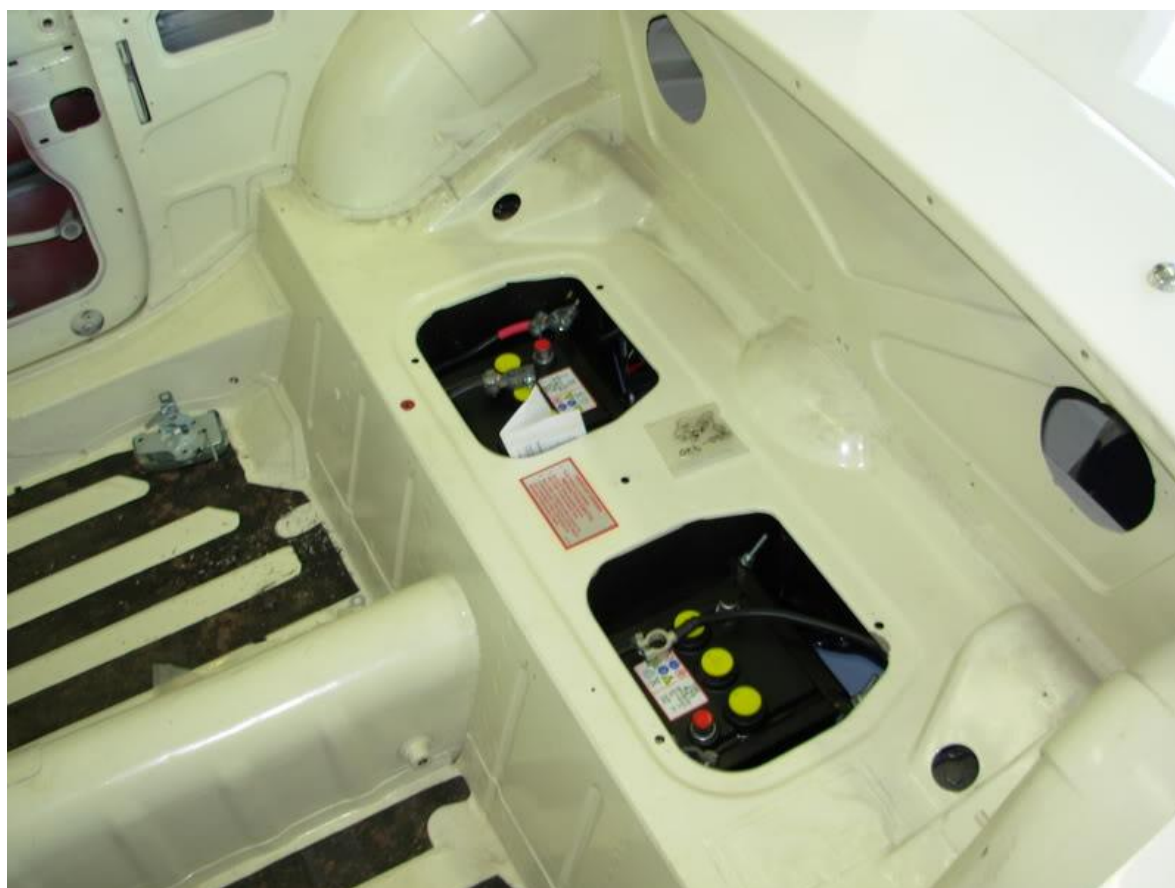
2x 6 volt batteries under rear compartment
