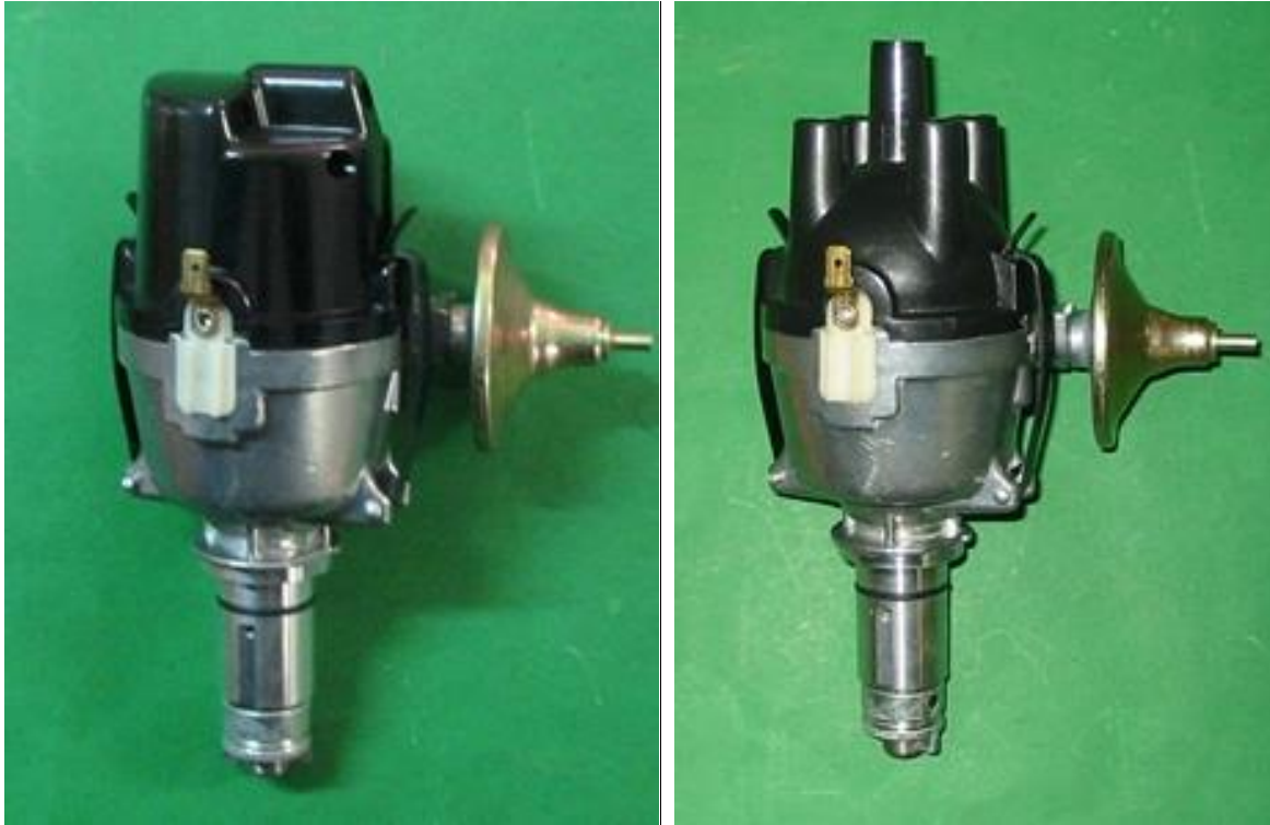
Lucas 25D distributor showing early side exit (18G,GA & GB) and later (18GD-) top exit
