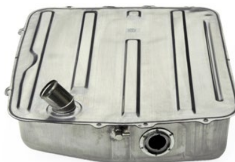
Later style fuel tank (screwed to underbody)
