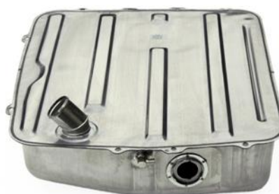
Later style fuel tank (screwed to underbody)
