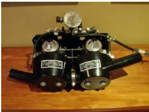
Photo showing air filters connected by balancing tube
