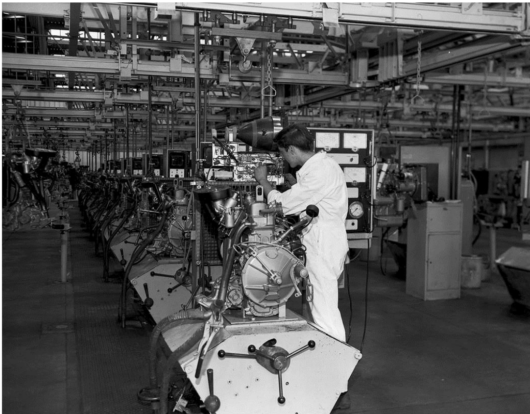
Hot Run station, showing setup. Note overhead delivery system.
