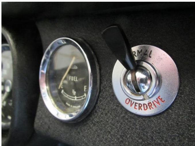
Overdrive switch and escutcheon (early type) (NOT USED IN AUSTRALIA)
