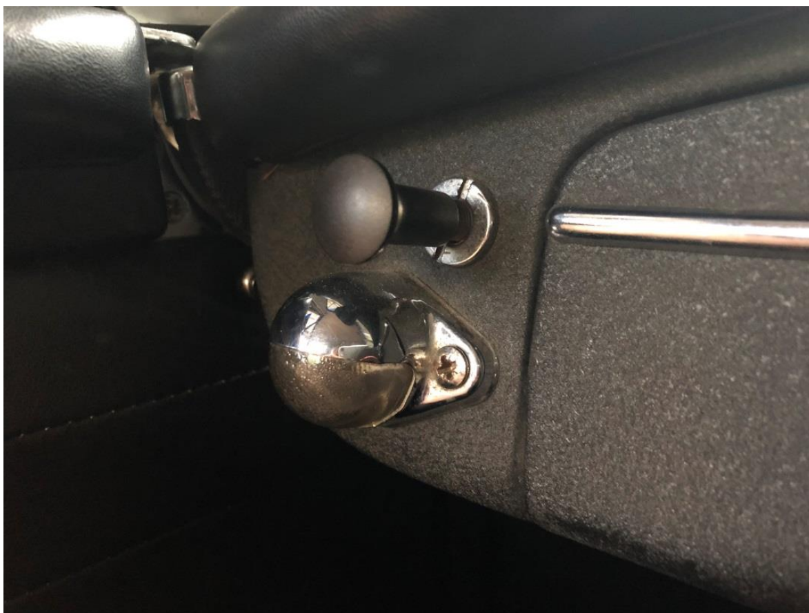
Map light and switch (Bakelite on this Mk I)
