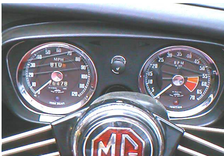
Mk 1 showing the rheostat switch. Note also the thin chrome strip around the inside of the instrument hood
