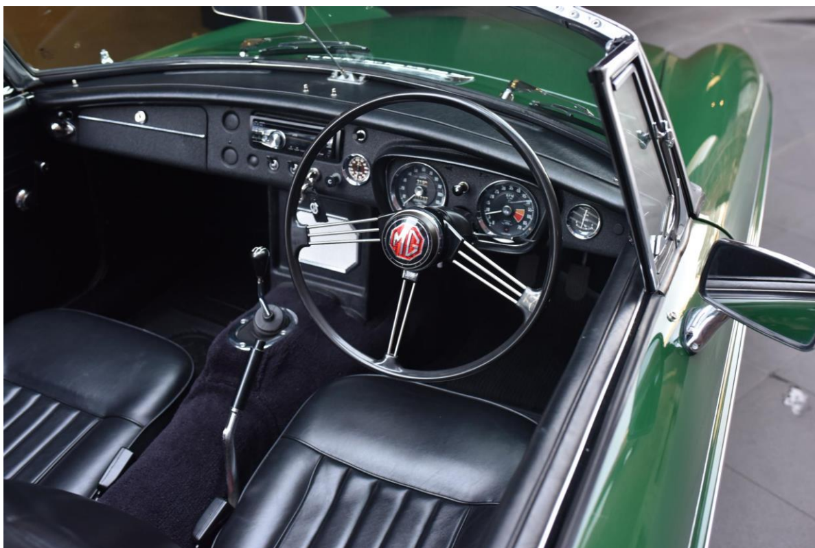
YGN3 719, clearly showing the early locations of the washer pump (above the oil/temp gauge) and the headlight toggle (next to ignition). Also note the 3 blanking plugs for heater (on left) and overdrive switch (on right).
