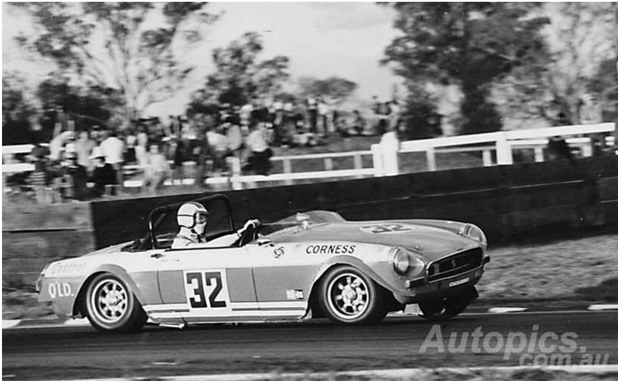
How we’ll always remember ‘the world’s fastest B’ at the peak of its development in 1971. Note the super lightweight ‘Minilite’ magnesium wheels from the UK were fitted by that stage, as the team focused on reducing weight in every area of the car.
