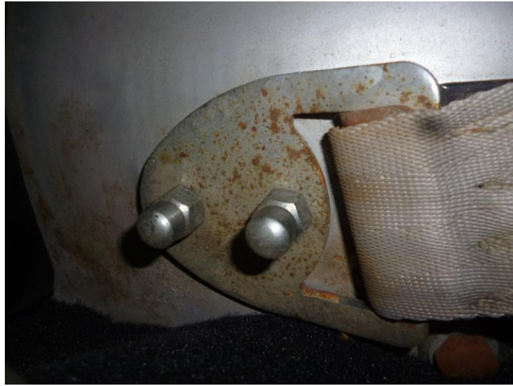
Typical BMC twin 5/16 stud anchorage (pre 1967)
