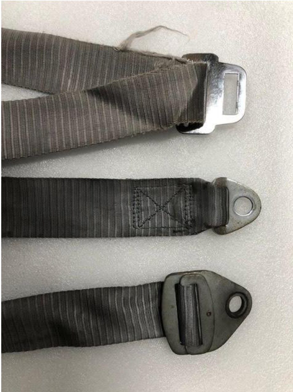
Single bolt mounting as fitted to later Mk I cars and all subsequent cars
