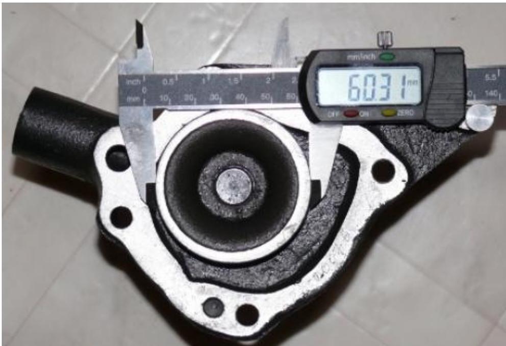
Impeller diameter and gasket face of GWP115, fitted to 3 main bearing MGB
