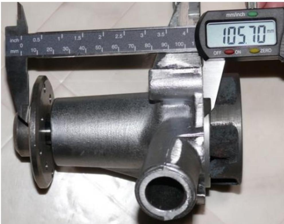
Length of GWP114, originally fitted 1965 to 1971
