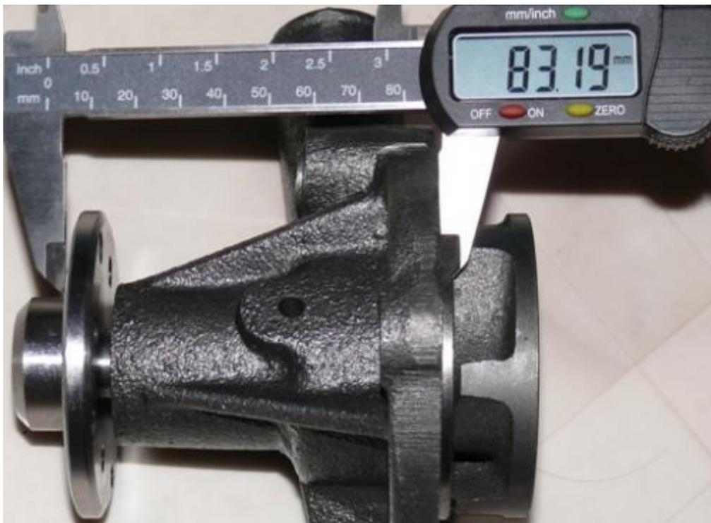
Length of late MGB 5 brg pump GWP130, originally fitted 1972 on
