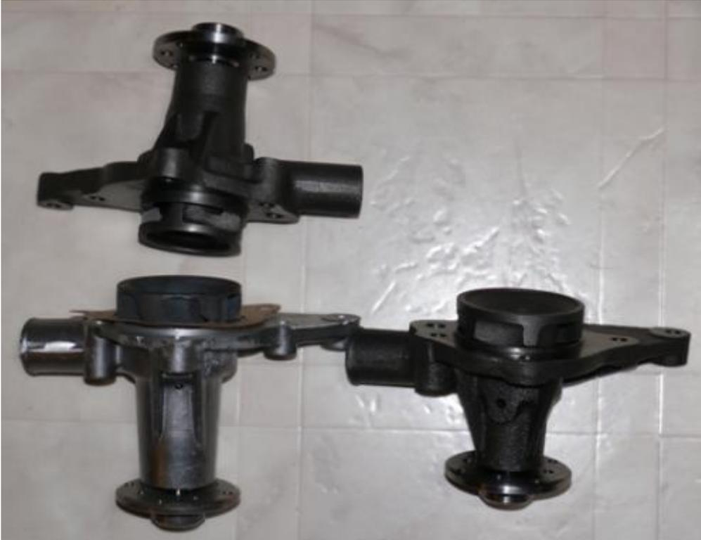
3 main bearing pump (top) has smaller impeller,GWP114 (lower left) is longer than GWP130 (right)
