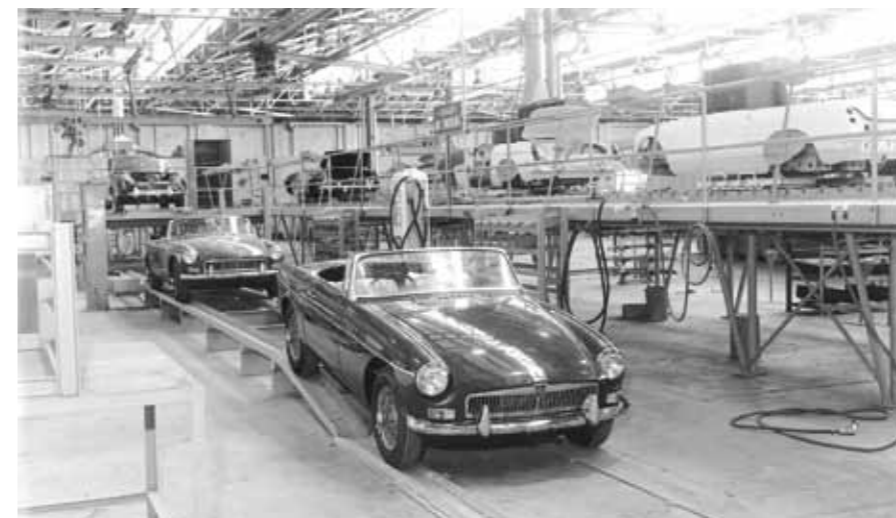
The first two cars off the Zetland line had to go through again. In the effort to outdo Abingdon production tolerances, the doors of these two cars were found to be jammed tight once the cars were lowered onto the ground!
