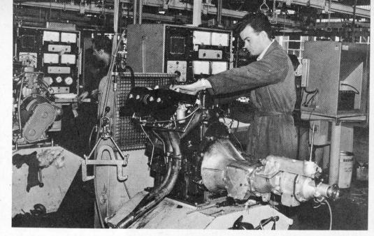
Left: In the Hot Run department, the MG engine is operated for a half-hour, during which time some 29 different checks are made to ensure everything is up to standard. Unlike most parts that go into the B, the engine/gear-box/overdrive unit is imported in fully assembled condition.
