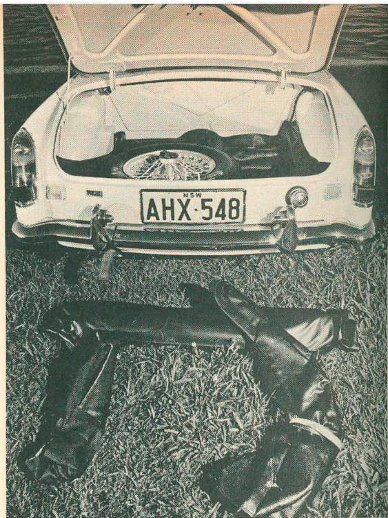
This is a photograph we haven't published before. It shows the amount of gear to stow into the boot when the hood is disassembled. There still remains a lot of boot space, and the area behind the two seats.
