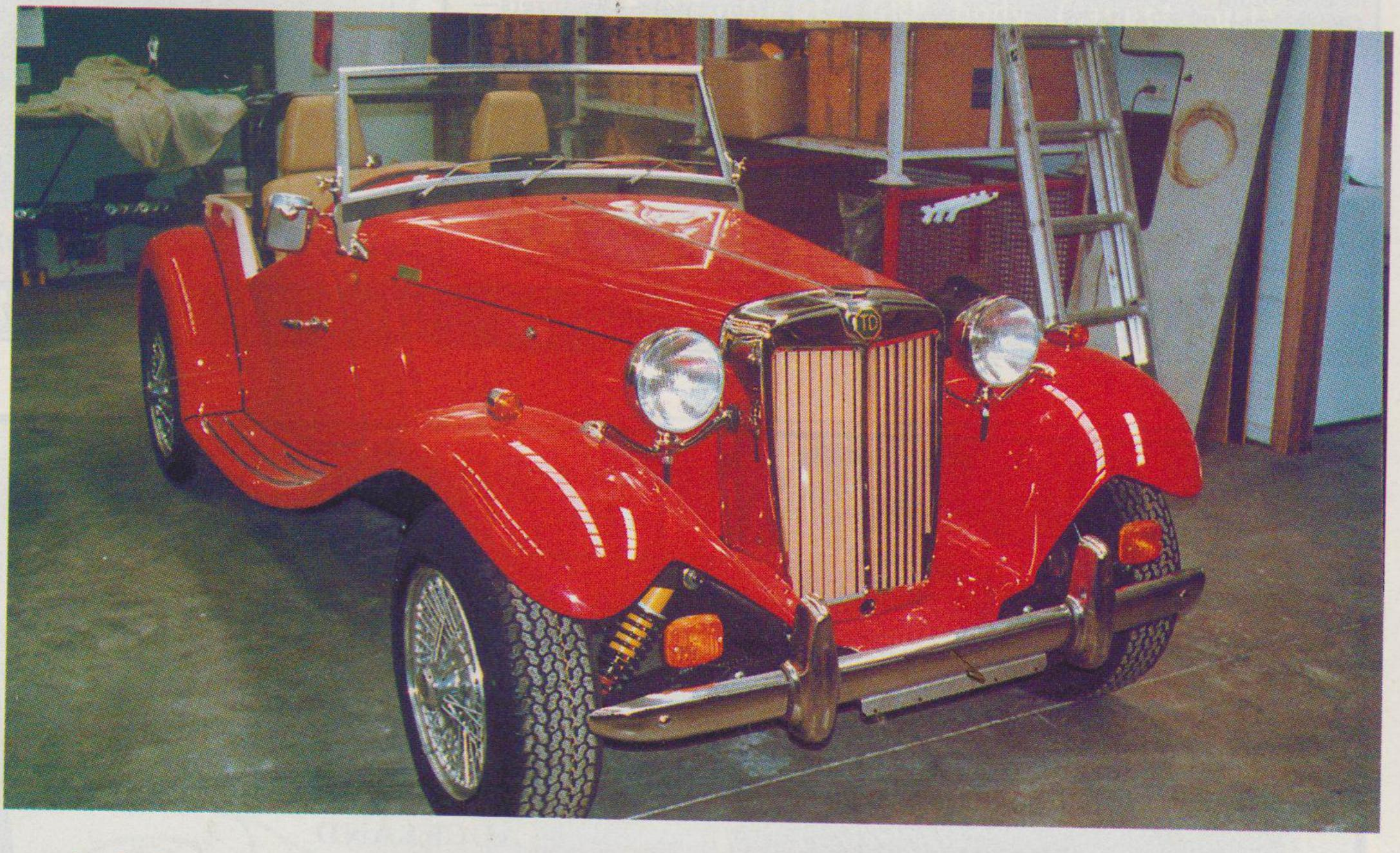
standard form, it will complete a standing 1/4 mile in 16.9 seconds, which compares more than favourably with the MGB (18.7s), 3.4 Mk2 Jaguar (19.1s) and 1275cc Mini-Cooper S (18.4s). Performance is assisted by the car's favourable power-to-weight ratio – although the TD2000 weighs a solid 900kg, it is propelled by an engine designed for a vehicle weighing almost half as much again.
