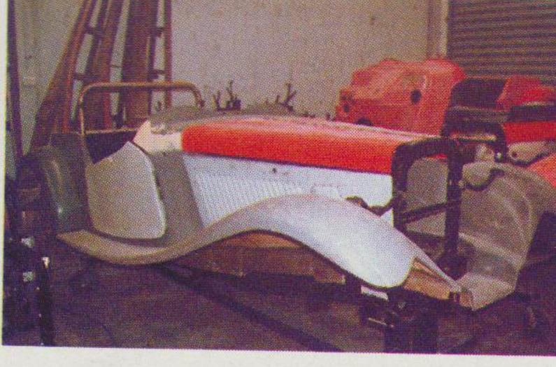
Left, body panels fully assembled to ensure fit, prior to painting
