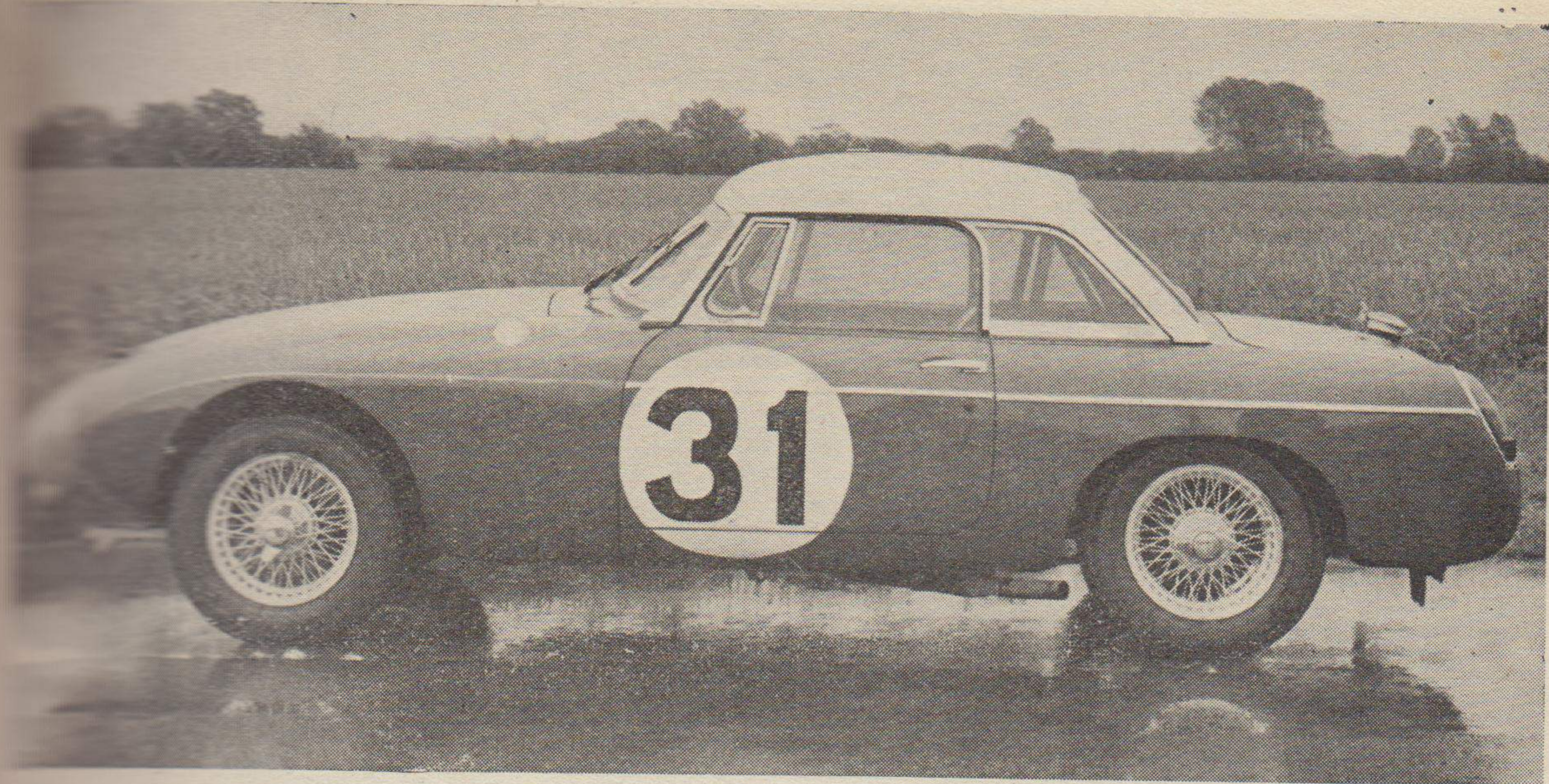
The sleek nosepiece and the well-designed hardtop gives the Le Mans B much better aerodynamic form than its normal production brothers.
