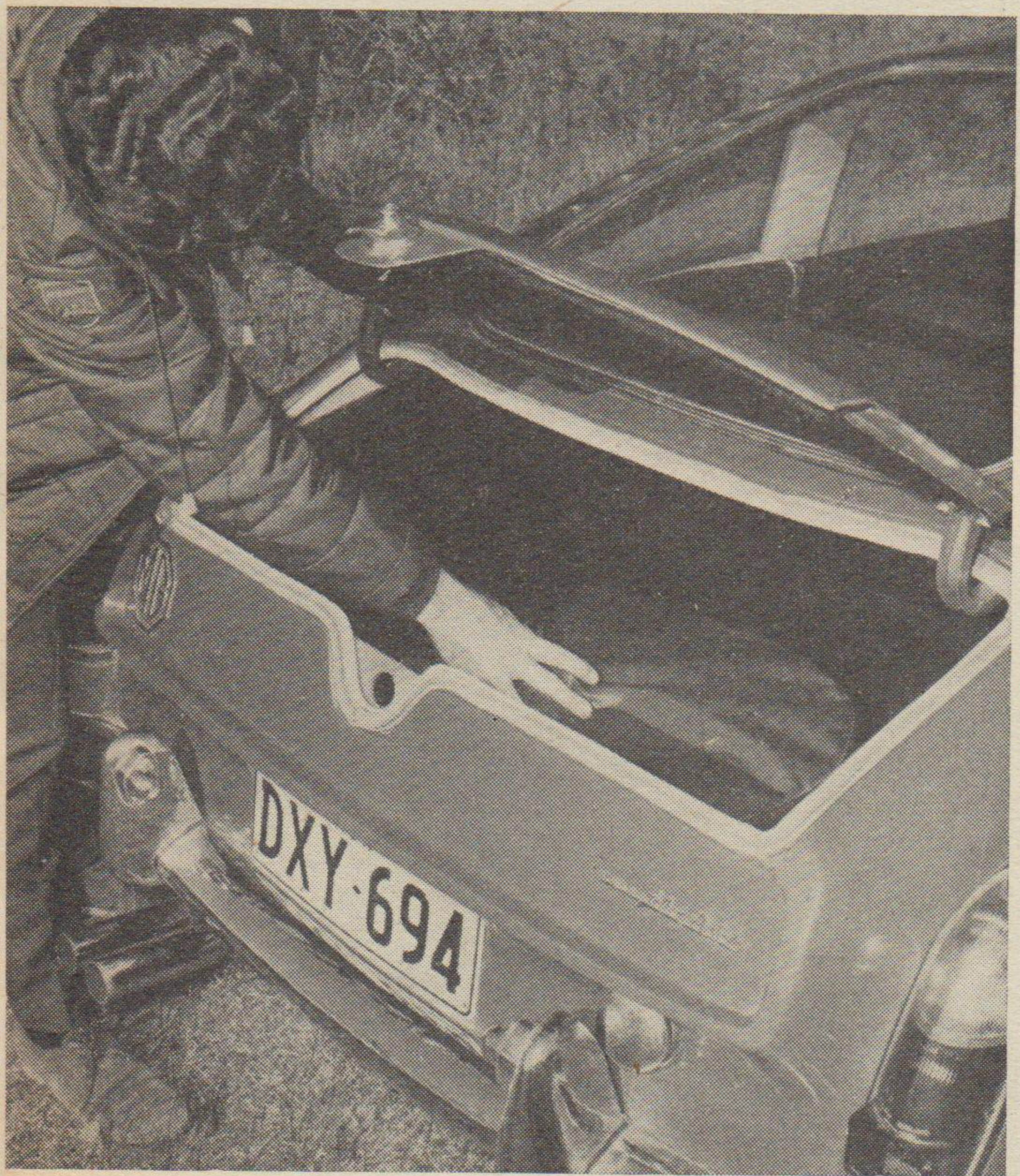
An inside look. Access to all compartments in GS car is through passenger's cockpit (seat is hinged). J and S has boot deck lid fitted — higher lip, deeper reach, slightly less space.
