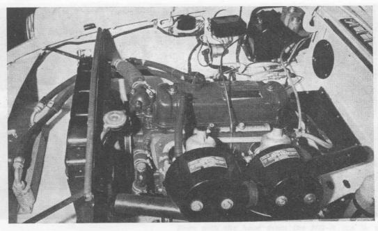
Engine is smooth and powerful. It is the BMC Bseries enlarged. Oil cooler up front is standard.
