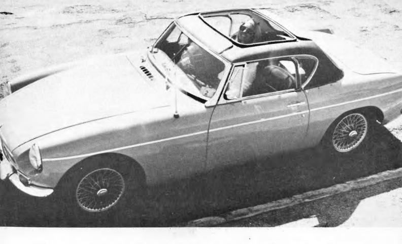
The J and S sunroof top is fitted to the car in a similar fashion to the standard hard-tops. When the top is removed it stows easily in the boot.
