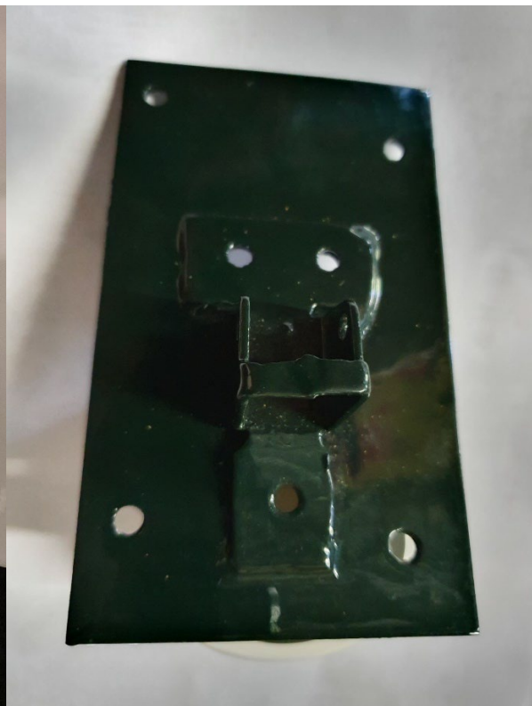
Catch plate welded to new plate
