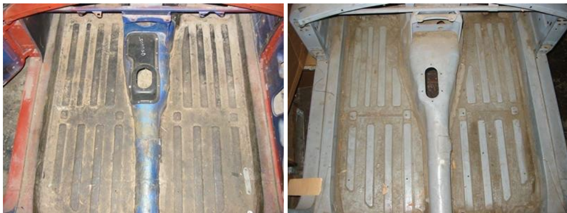
Figure 1 Early 3-sync tunnel c/f wider 4-sync tunnel. Compare the ribs on both sides to see the difference.
