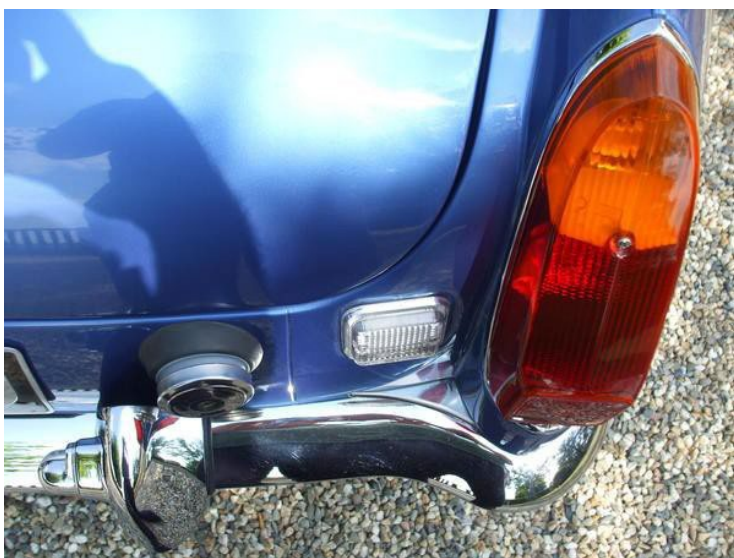
Later smaller bumper infill (polished alloy)
