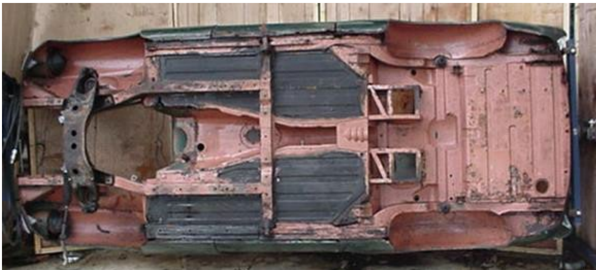
Photo showing monocoque construction (photo: mg.net)
