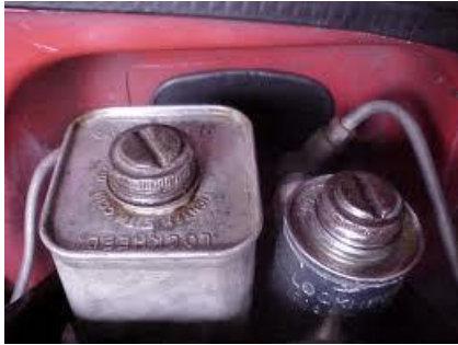
Master cylinder + different caps
