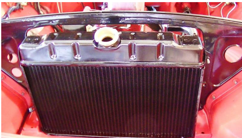
Later style radiator with central refill access
