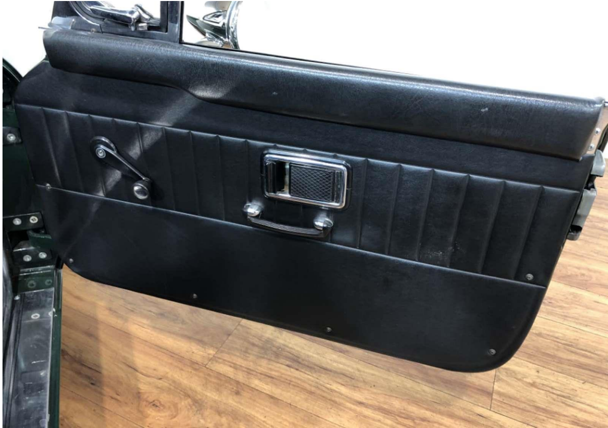
Mk II Door card with 'ladder' pattern
