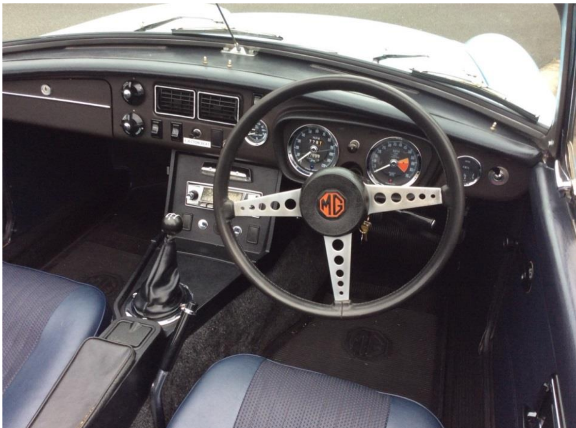
Photo showing MGBL (facelift) with air vents (11). Note: rocker switches instead of toggle, new console with radio, map light above radio, toggle switches or blanks. Also note new seat design (blue), arm rest and ash tray, temp gauge in C-N-H, steering wheel and column ignition/steering lock.
