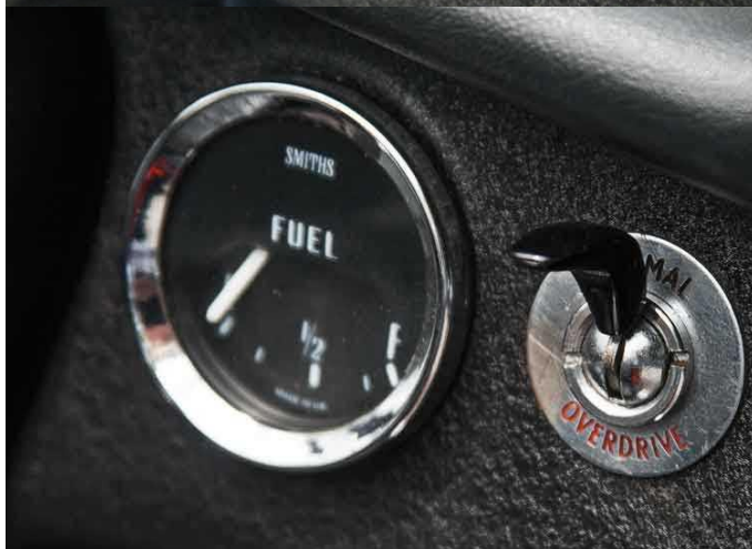
Later style 'hooked' overdrive switch . (ALL Australian overdrive switches should be of this type.)
