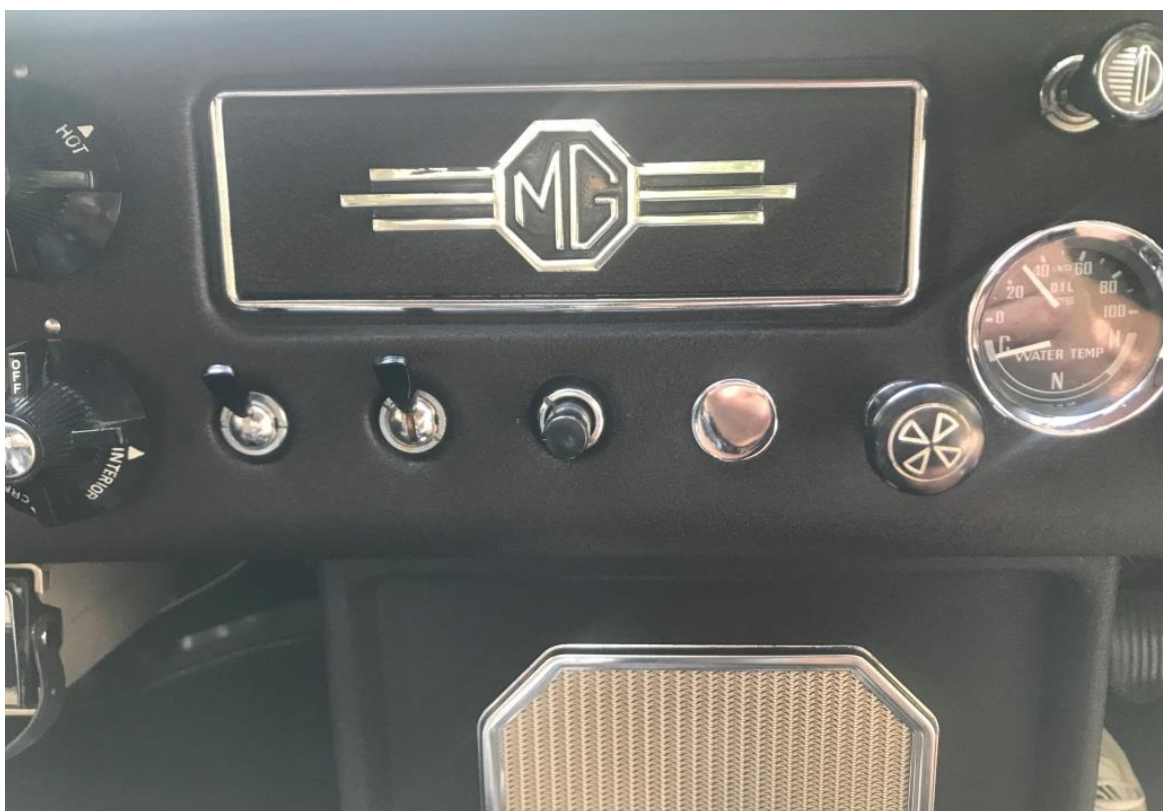
1970 MGBL showing heater controls (just), toggle switches, washer pump, chrome ignition blanking plate (that is not a blob of chewy – it's the reflection of the photographer's finger), later style choke knob, later style headlight switch, temp (C-N-H) & radio blanking plate.
