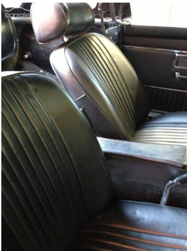
First BL seats with headrests. Also just visible is chrome reclining lever
