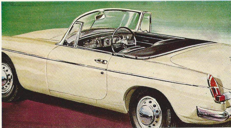
This picture illustrates the fold-away type hood available as an optional extra to form a convertible model, neatly stowed in the space behind the front seats.
