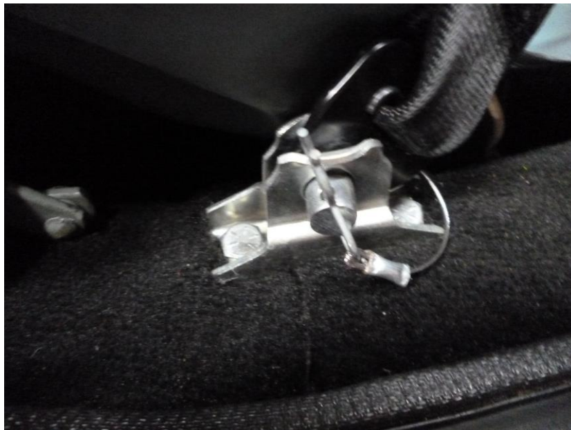
Later MGA door-step belt (detachable) anchorage
