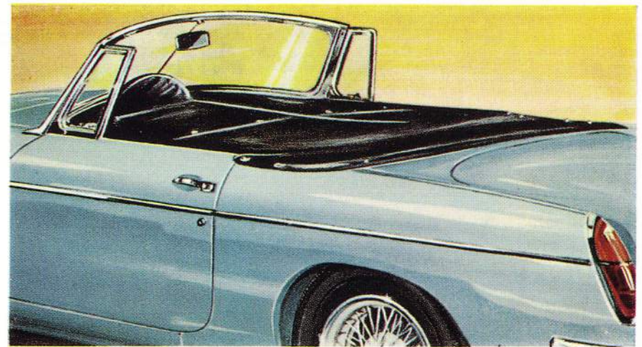
The optional extra tonneau cover is shown here. The provision of a zip fastener enables the driver to use the car without detaching the tonneau completely.
