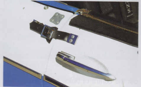
Strap on door for added safety.
