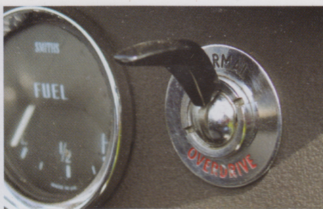
This overdrive switch was common to all Aussie-built MGBs with overdrive.
