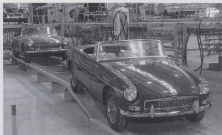
Early assembly at Waterloo. Note the indicators outboard of the parker lights.
