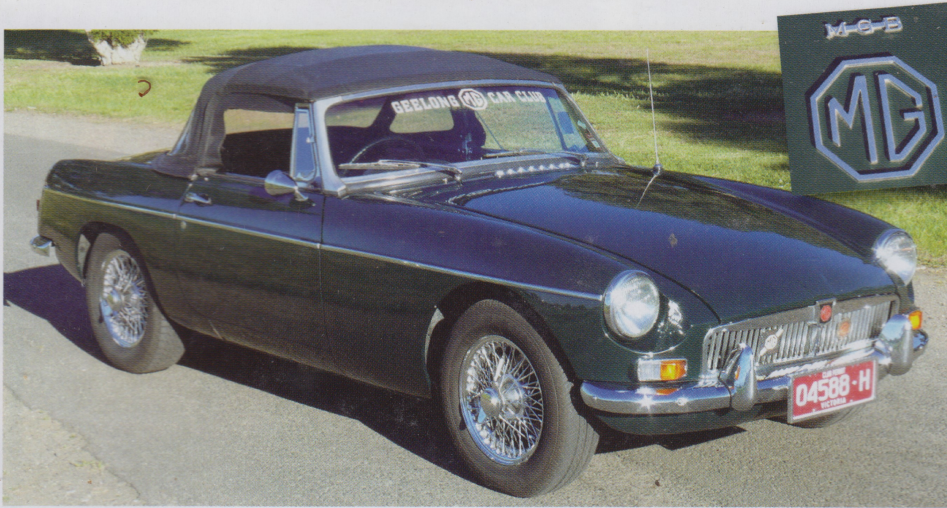
Early Enfield-built MGBs feature pull door handles, pack-away roof and chrome grille.
