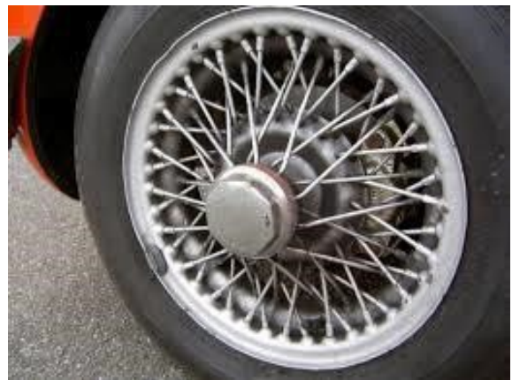
Mk II standard, painted wheel ( with octagonal knock-on)
