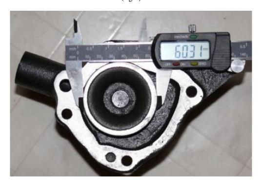
Impeller diameter and gasket face of GWP115, fitted to 3 main bearing MGB
