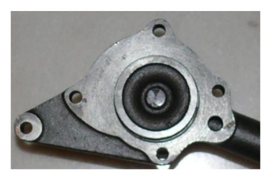
MGA pump has same 60.3mm impeller diameter as 3 brg B but different bolt pattern
