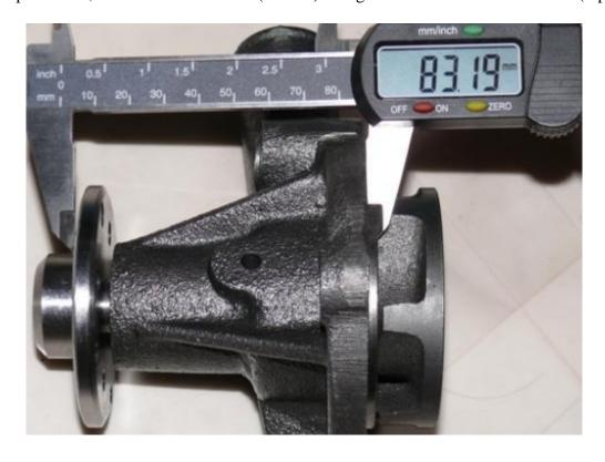
Length of late MGB 5 brg pump GWP130, originally fitted 1972 on
