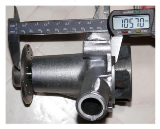
Length of GWP114, originally fitted 1965 to 1971
